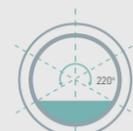
Rigid conduits are perforated at  $220^\circ$
